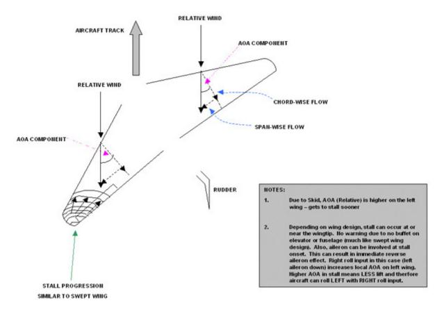
This diagram helps try and illustrate the differences in AOA when the aircraft is in a left skid.
